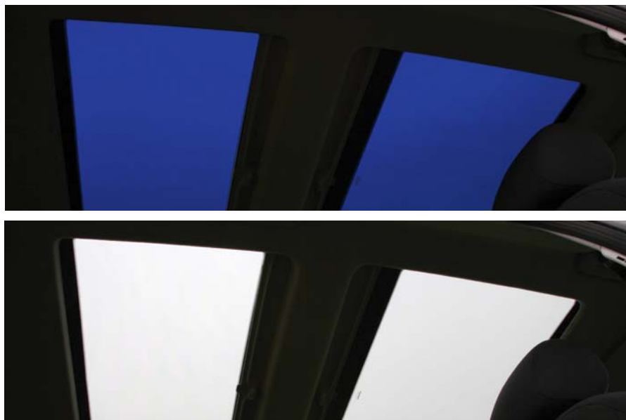
Shown fitted in a car roof rack, Pilkington Sundym Select™ can be switched instantly from clear (bottom) to tinted (top) mode.
